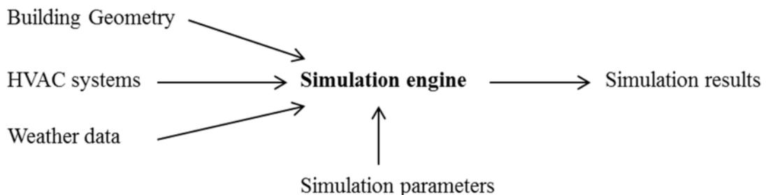
Figure 3 Input/output data of thermal simulation engine
